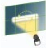
Contrast R + Refractor N°2 (Glass with wide angle asymmetrical beam)
